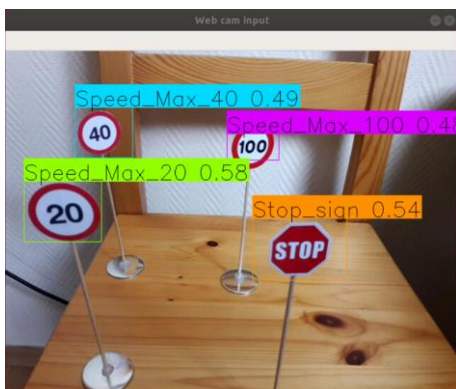
Figure 7. Testing the model under well-lit conditions
